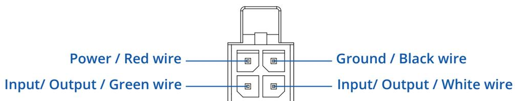
I/O (PIN 3 and 4): Configurable digital Input/Output pins. Open collector output, max output 30 V, 300 mA or Digital input where 0-6 V detected as logic low and 8-30 V - logic high
