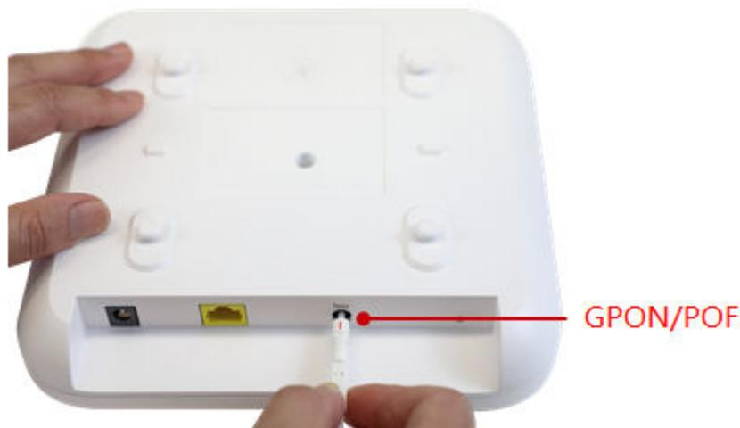
**Figure 6-3** Removing a PoF cable
