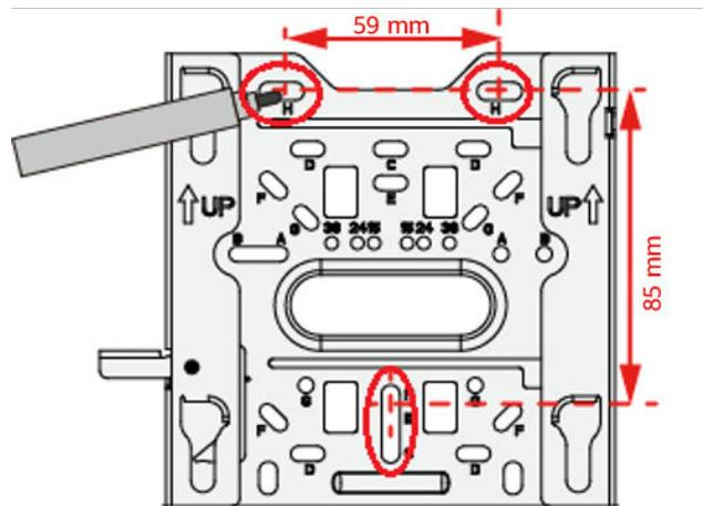
2. Use a 6 mm drill bit to drill 40 mm to 45 mm deep holes in the marked positions. Hammer the expansion tubes into the holes until the expansion tubes are flush with the wall.
