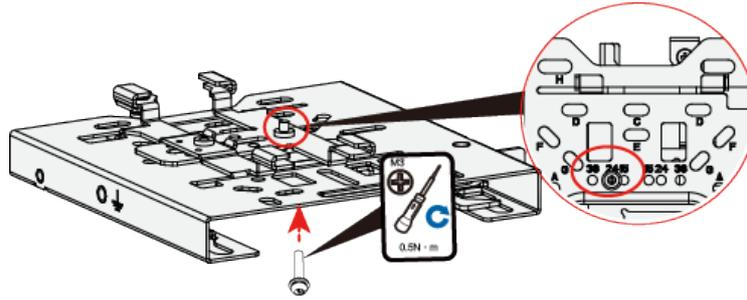
5. Insert mounting bracket a into the T-rail, and slide mounting bracket b along the slot until the T-rail is tightened.
