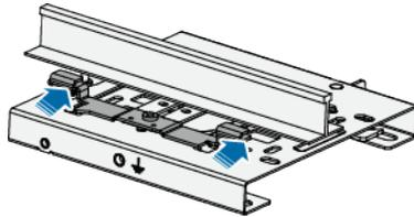
6. Secure the M3x8 screw through hole 24 marked in the following figure, and secure T-rail mounting bracket b. Tighten the M3x6.2 set screw for installing the T-rail mounting bracket.
