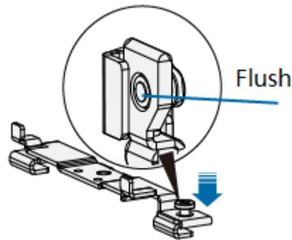
3. Install the flat-edge T-rail mounting brackets a and b along the sliding slot on the mounting bracket body in the sequence shown in the following figure.
