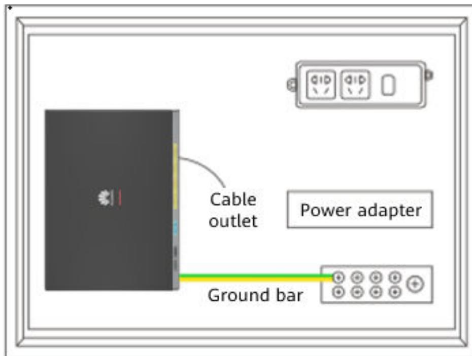
**Figure 3-2** Vertical installation diagram
