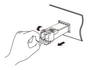
4. Reinstall the protective dust plug in the SFP's optical bores and place it on antistatic mat or a static shielding bag.
